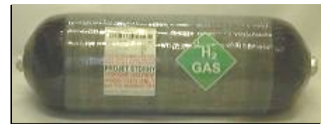
Type IV, 700 bar industrial prototype
