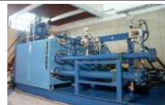
Hydraulic set-up for cyclic tests
