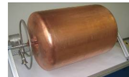
Prototype of the inner tank with hydrogen permeation barrier made of coated copper on the composite outer surface
