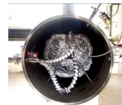
Prototype inner tank with thermal insulation after integration in a cryostat for liquid hydrogen tests at minus 253 °C
