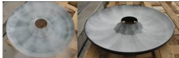
Inner tank dome during and after the thermo-shock test with liquid nitrogen
