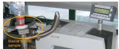
Sample mounted on spectrometer for permeation measurement
