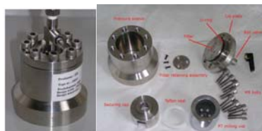
One of the in-house built high-pressure milling vials
