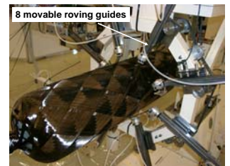
Optimized prototype (stiff steel frame)
