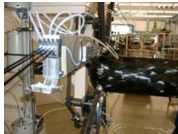
Final construction with resin dosing system during vessel winding (CF/EP, aluminum liner)
